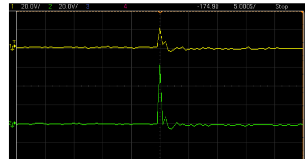
Fig 3: Time domain pulse captured by different antenna configurations using oscilloscope at a voltage scale of 20 Volts/Div and time scale of 5 microsecond/Div.
