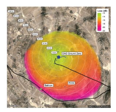
Three "Heliotrope" solar-heated balloons were launched earlier in the day. The structure of the atmosphere creates alternating ensonified and acoustic dead zones as infrasound rays refract and internally reflect, shown by raypaths in the figure on the right. While two balloons were outside the ensonified zone capable of detecting an arrival from the explosion, a third balloon was at the edge of the ensonified zone at 20 km altitude and 56 km away from ground zero.
