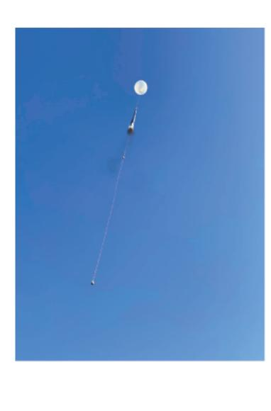
The 2021 BASS campaign was conducted between July and September. A total of 38 heliotrope balloons were launched, 26 of which reached float. The balloons were equipped with two barometers on a tether. This configuration allows for signal stacking and time-of-flight correlations to determine the arrival direction of the signal. The entire campaign was student-led and operated under the guidance of staff from JPL, Sandia National Laboratories, and Oklahoma State University.
