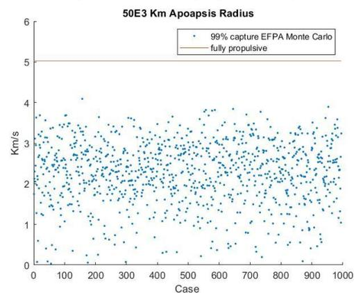
Figure 1.  $\Delta V$  needed post Aerocapture
