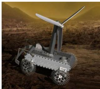
**Figure 1.** Wind-powered rover concept for potential Venus mission [1].
