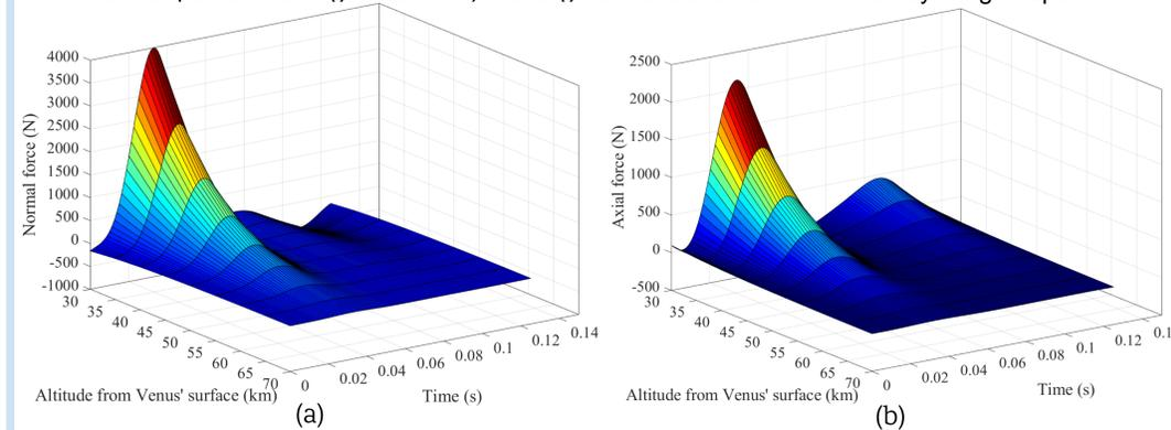
**Figure 3.** (a) Lift force and (b) drag force of flapping wing drone on Venus from 30 km to 70 km.
