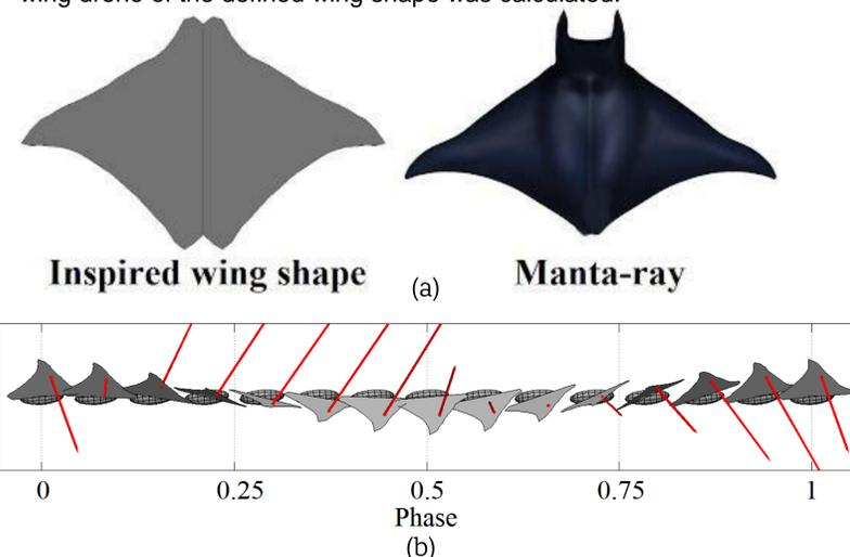
**Figure 1.** (a) Wing shape used for aerodynamic analysis of a manta ray bio-inspired drone and (b) visualization of one cycle of flapping wing drone's flight progression.
