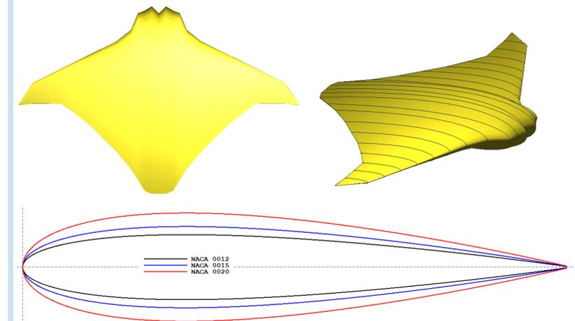
**Figure 2.** Model of fixed-wing drone in XFLR5.
