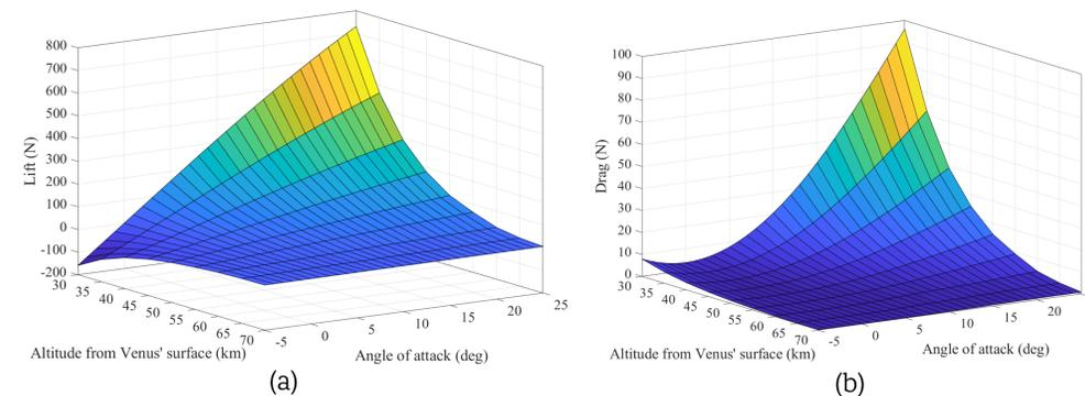
**Figure 4.** (a) Lift force and (b) drag force of fixed-wing drone on Venus vs. angle of attack from 30 km to 70 km.
