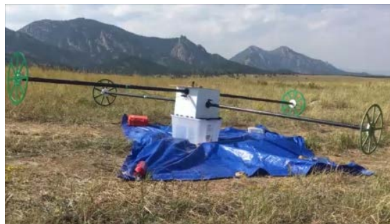
Fig. 2. BTEM outdoor ground test near Boulder. Electric fields are measured between boom-tip electrodes; magnetometers are inside booms.
