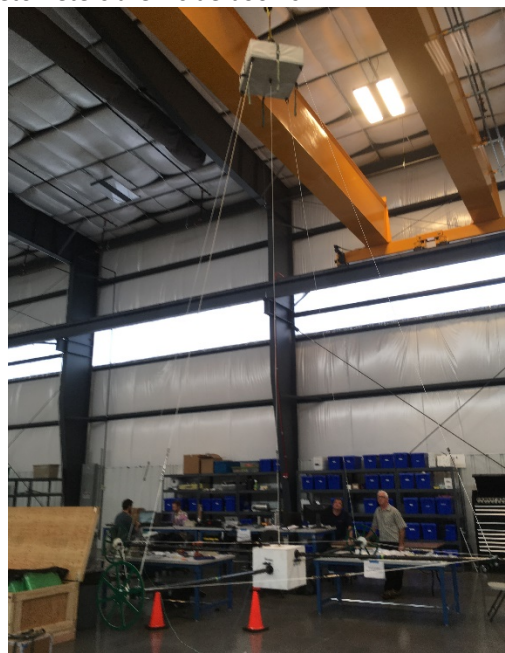
Fig. 3. BTEM (above cones) rigging test beneath balloon avionics package (near ceiling) at World View high bay. Separation mitigates potential interference from continuously operating radio systems.
