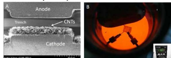
**Figure 1: (A) SEM image of CNT diode (B) InAlN/GaN devices operating at 700 °C.**
