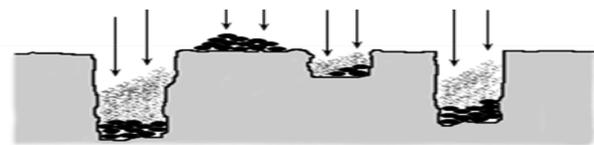
**Fig. 3.** UV can be attenuated by multi-layers of cells or by UV absorbing dusts, greases, etc. (adapted from Schuerger et al. [16]).
