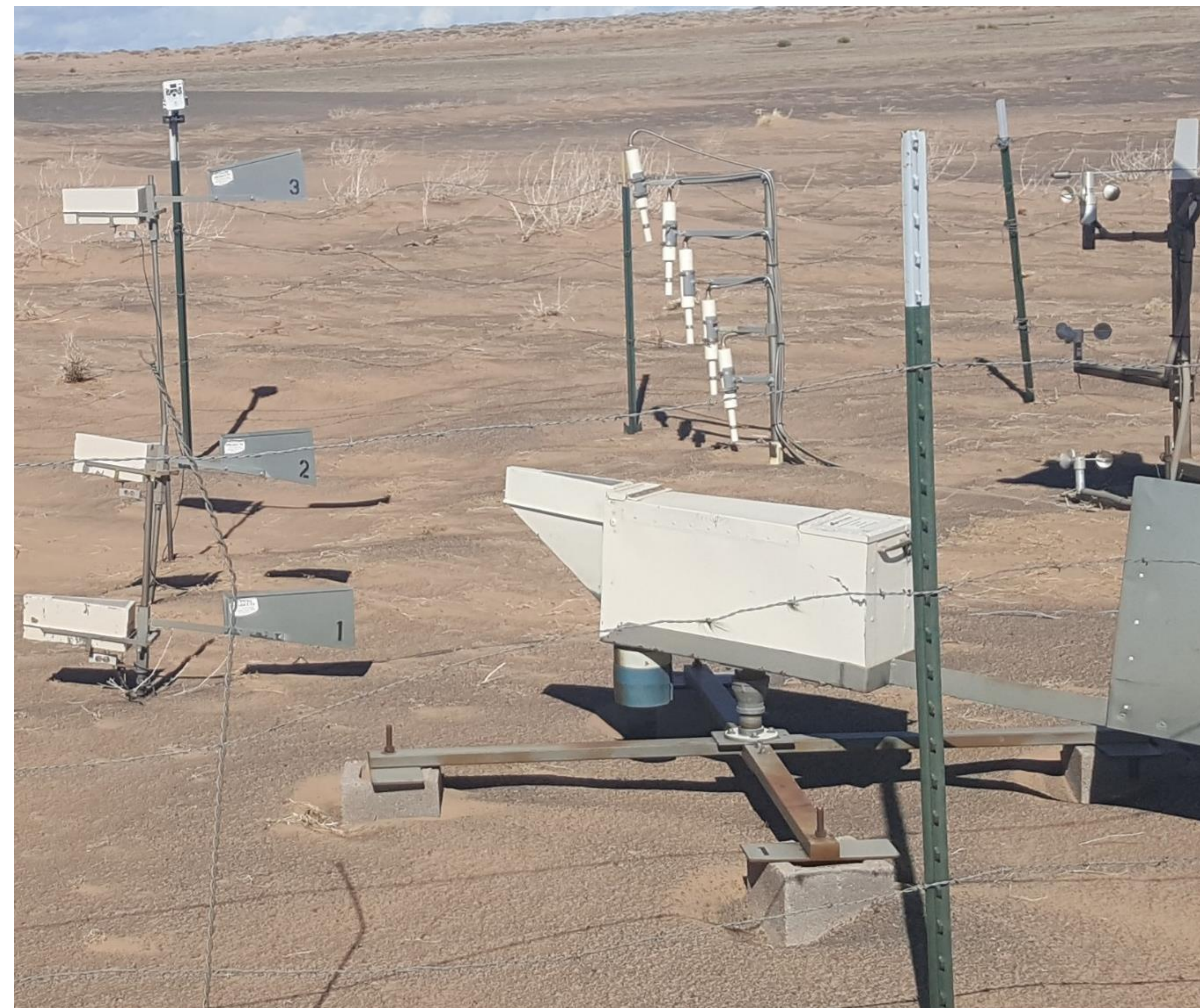
Figure 1: The suite of instruments to measure horizontal mass transport (HMT) are shown with the BSNEs on the left, the saltation sensors in the middle and the anemometers on the right. In the center foreground is a fourth BSNE that monitored sediment volume.
