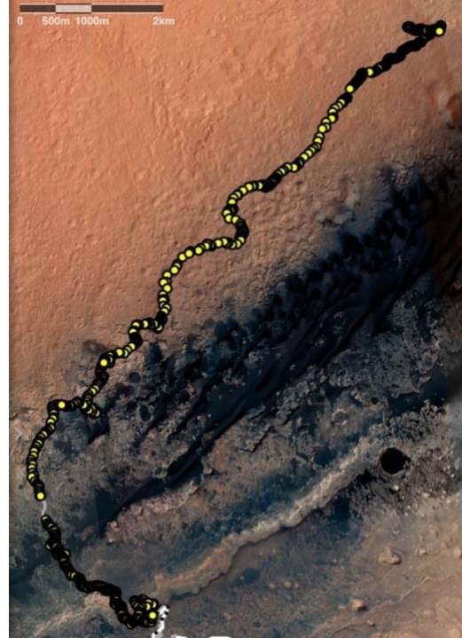
Figure 1. Example of 2,940 unique Mars Science Laboratory's DAN (Dynamic Albedo of Neutrons) Instrument science observations at 822 rover locations throughout 2,333 sols localized to the MSL mission HiRISE basemap.
