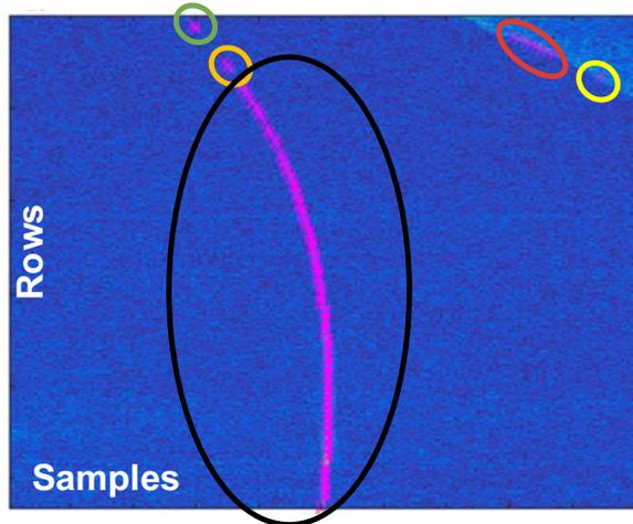
Figure 1. Signal estimated locations. Similarly structured noise causes false estimates in the upper right. MSMR segments are shown as ellipses.
