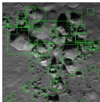
One of the outputs of the feature detector is an image with detections labeled with bounding boxes. The image to the right shows a closeup of result image M109309907LC, where detected rocks are labeled with green bounding boxes.
