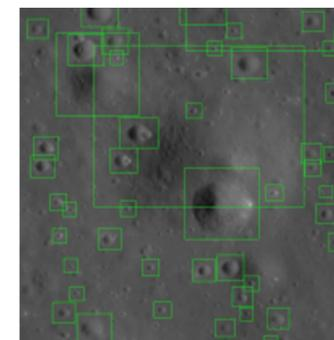
Result close-up of crater detection using the feature detector on image M114131846RC. Craters are labeled with green bounding boxes.
