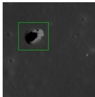
Feature detection of a single lunar pit on image M184068107LC, labeled by a green bounding box. There are few known lunar pits, and many craters. The feature detector successfully distinguished between the two.
