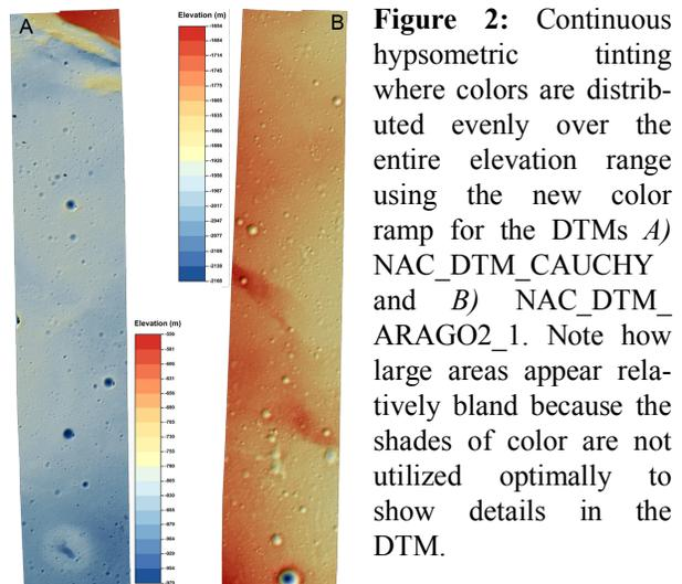
**Figure 2:** Continuous hypsometric tinting where colors are distributed evenly over the entire elevation range using the new color ramp for the DTMs *A*) NAC\_DTM\_CAUCHY and *B*) NAC\_DTM\_ARAGO2\_1. Note how large areas appear relatively bland because the shades of color are not utilized optimally to show details in the DTM.
