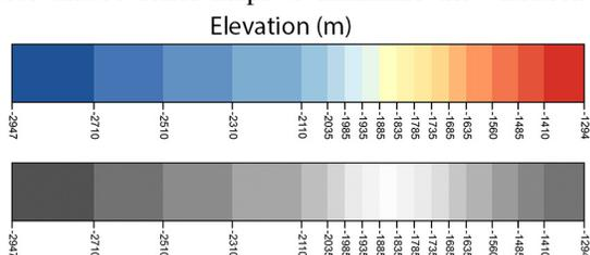
**Figure 3:** An example of a color legend from the new color ramp in both full color (top) and in grayscale (bottom). Note that both versions are perceptually linear, with the color version proceeding from cool to warm colors and both versions increasing in luminance towards the center of the diverging color ramp.
