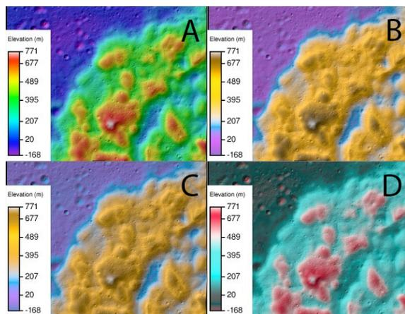
**Figure 1:** Rainbow color-shaded relief of the Apollo 16 landing site (NAC\_DTM\_APOLLO16) and the accompanying legend in *A*) common, *B*) protanopia *C*) deuteranopia and *D*) tritanopia vision simulations [8]. Also note how the luminance of yellow (~489 m elevation) creates an artificial contour in *A*. There is a similar effect in *C* and *D*.
