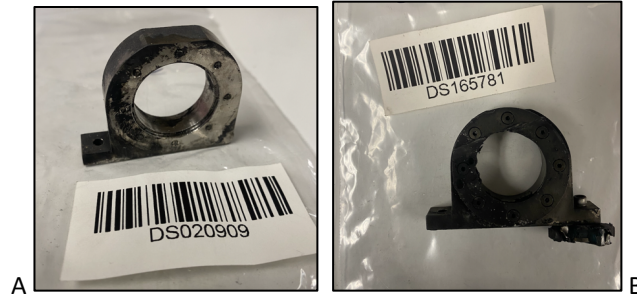
Fig. 6. Titanium Camera Mounts After HVI
