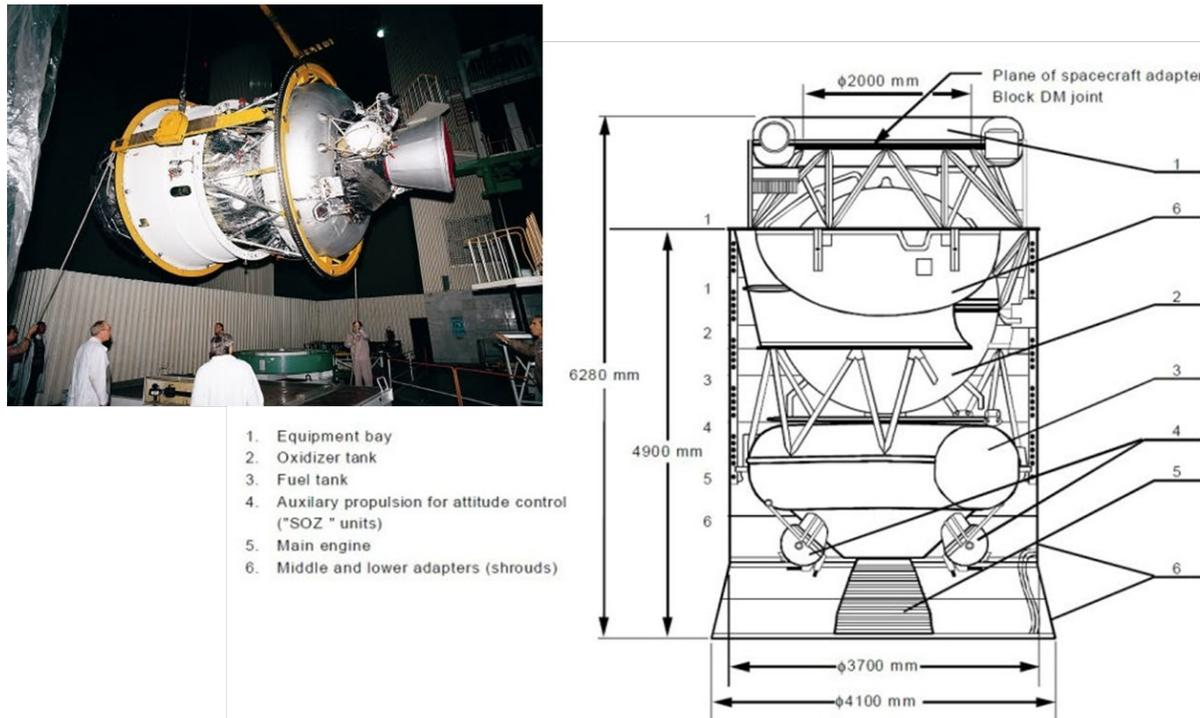
Fig. 1. Photograph and Line Drawing of the SL-12 Fourth Stage Rocket Body.
