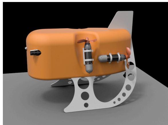
Figure 1. Engineer rendering of a new full-ocean depth autonomous underwater "drone" vehicle, capable of examining deep-ocean ecosystems via multiple landings and transits on and over deep ice-covered and hadal seafloor.
