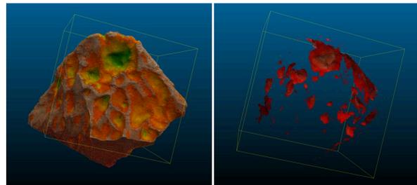
Figure 4. Regmaglypts and other surface hollows from atmospheric ablation can be characterized and isolated digitally on terrestrial analogs, as illustrated here with the 12.7 kg iron meteorite Bruno. Bruno exhibits classic regmaglypt and associated flow structures with striated fusion crust. Center for Meteorite Studies specimen.
