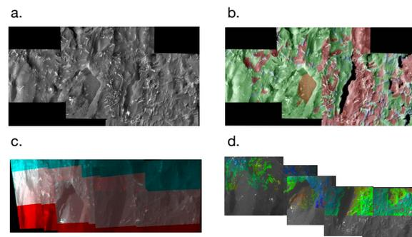
Figure 2. The New Shoreham Microscopic Imager dataset has been revisited to produce anaglyphs and Micro-Digital Elevation Models using respective MI frame stereo pairs. The original mosaic (a) has been mapped to reveal oxide coating coverage, bare metal surfaces, and expressions of the Widmanstätten pattern (b). (c) stereo anaglyph mosaic. (d) preliminary micro-DEM coverage. North is the right; width is approximately 12 cm. Image credit: NASA/JPL/MI/MIPL.
