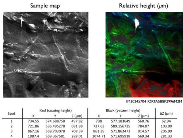
Figure 3. Example of Widmanstätten pattern within the New Shoreham MI mosaic showing details at the micron scale using MicroDEM examination. Height measurements of the resistant plates (likely either taenite or schreibersite) and the surrounding coating confirm the cross-cutting relationship inferred visually in [5]; see table inset.
