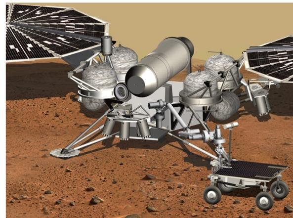
Figure 2: Notional artist's concept of transfer of sample tubes from the Sample Fetch Rover to the Sample Retrieval Lander, using the Sample Transfer Arm on SRL to load the sample tubes into the Orbiting Sample container on the Mars Ascent Vehicle
