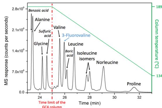
**Figure 2.** Gas chromatogram obtained with a spare GC4 column of a 22 amino acids standards mixture analyzed in the laboratory. Only alanine and glycine would be detectable within the current SAM-flight operating conditions used for the GC4 column on the SAM flight model instrument. However, this laboratory experiments shows that recording the signal while the temperature is cooling down on Mars could allow the detection of heavier molecules such as the amino acids targeted for this study.
