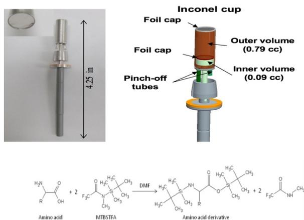
**Figure 1.** The MTBSTFA derivatization cup (top) and an example of the MTBSTFA reaction with an amino acid that displaces the labile hydrogens with a *tert*butyldimethylsilyl group to produce a volatile amino acid derivative (bottom).
