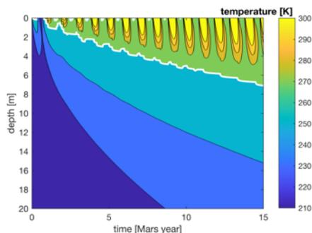
**Figure 5.** Simulated warming underneath a solid-state greenhouse habitat on Mars. Contours show temperature vs. time in an ice-rich regolith underneath a 2.5-cm silica aerogel layer on Mars in the Arabia Terra / Deuteronilus Mensae region (40N, 340W).
