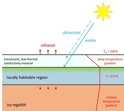
**Figure 1.** Schematic of the silica aerogel solid-state greenhouse habitability concept for Mars. A thin translucent layer of low thermal conductivity material transmits visible light but blocks ultraviolet and infrared, directly replicating the radiative effects of Earth's atmosphere.
