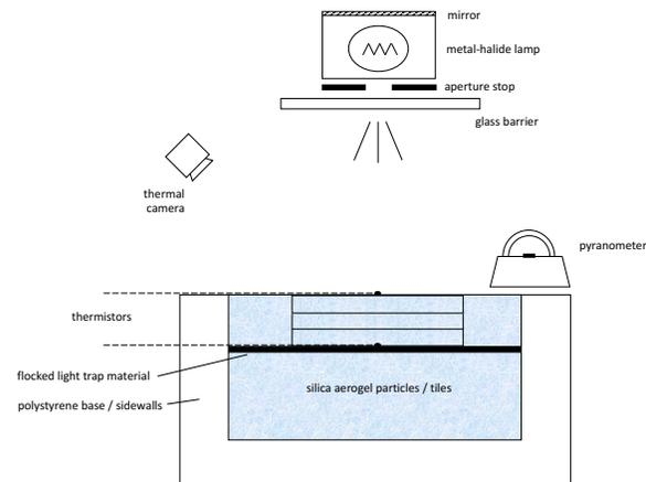
**Figure 3.** Schematic of the experimental setup.
