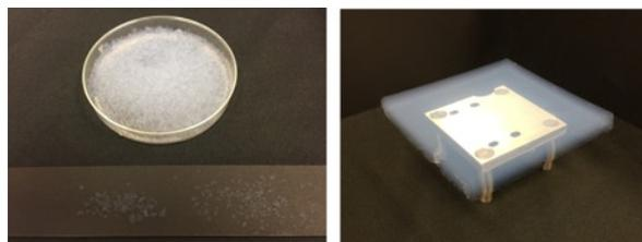
**Figure 2.** Image of the silica aerogel used in the experiments. (left) Silica aerogel particles with radii between
