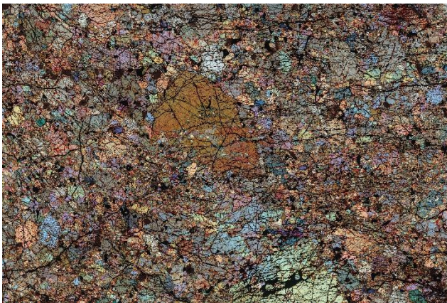
Figure 1. Partially cross-polarized optical thin section image. Note the unusually large olivine grain at center. Width of field = 23 mm. Image © Neil Buckland.
