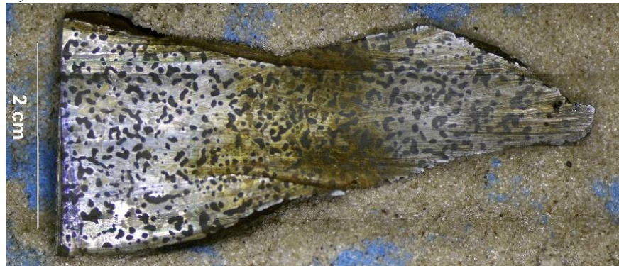
Fig. 1: Cut surface of Sirjan 001. Troilite (dark) and Fe-Ni (grey) are the main components of this meteorite.
