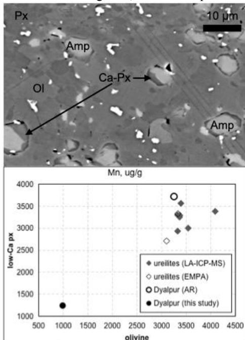
Fig. 1 BSE-SEM image and Mn content in olivine and pyroxene.
