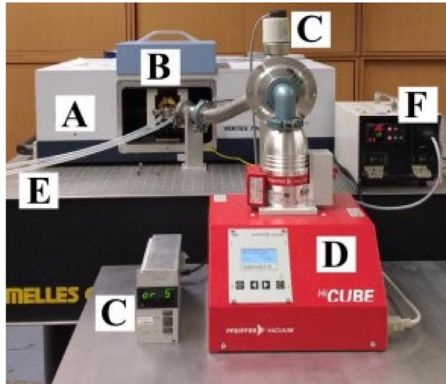
**Fig.1:** The Harrick Heating Stage and Praying Mantis set-up in the IRIS lab in Münster. (A) Spectrometer with detector; (B) Praying Mantis with sample chamber; (C) Vacuum gauge head and corresponding controller; (D) Vacuum pump; (E) Flexible tubes for water cooling system, which cools the housing of the sample chamber; (F) Heat controller.
