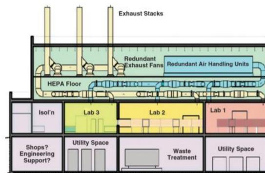
**Figure 4:** The Mars Sample Receiving Facility plan proposed by the Flad and Associates group, reproduced from Beaty et al. (2009)
