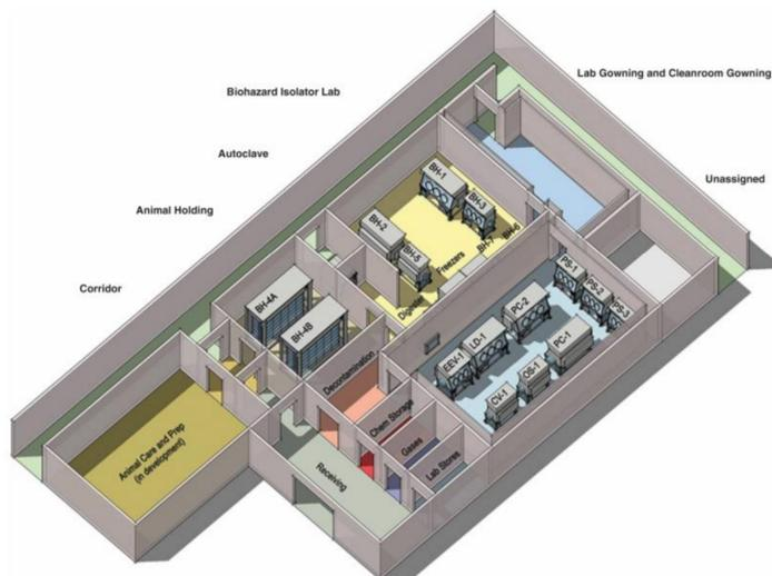
**Figure 2:** The Mars Sample Receiving Facility floor plan proposed by the Industrial Design and Construction group, reproduced from Beaty et al. (2009)
