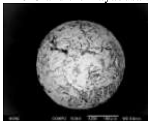
Figure 1. Electron-micrograph of FeC-bearing spherule formed by quenched process from the Nio meteorite shower in air, which has been collected by magnetic separation method at impact site of the Nio rice-paddy soils.
