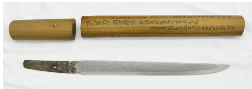
Fig.1. Photograph of Ryuseito . A tree-like pattern is observed on the surface of the blade. The full length of the sword is ~30cm.
