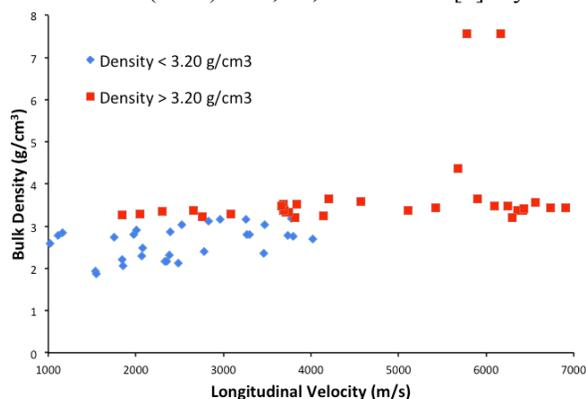
**Figure 1.** Relationship between longitudinal velocity and bulk density. Density must be above 3.20g.cm<sup>3</sup> for velocities faster than 4100 m/s.
