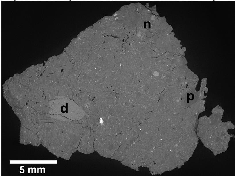
**Figure 1:** X-ray tomograph slice through the sample of NWA 11421. Lighter tone indicates greater X-ray attenuation (i.e., average atomic number). Brightest spot at lower center is likely sulfide or metal. ‘d’ is the dunite clast. ‘p’ is a fragment of plagioclase. ‘n’ is a clast dominated by pyroxene and plagioclase, with a little olivine – likely a norite.
