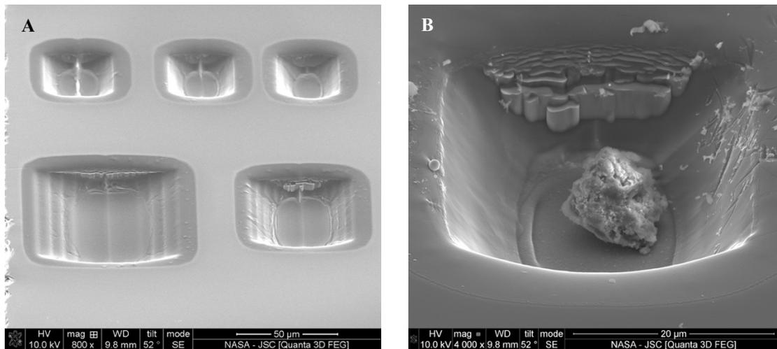
Figure 1: A) Particle wells produced via FIB milling. B) Secondary electron image of 10 $\mu\text{m}$  particle in well.
