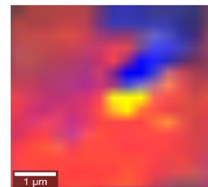
Fig. 3 Raman map displaying the distribution of elemental sulfur (yellow), augite (blue) and hematite (red). Brightness represents intensity.
