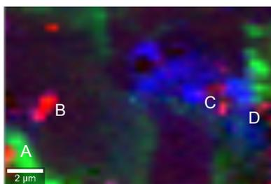
Fig. 1 Raman map of MMC (red), labradorite (green) and augite (blue) is displayed. Brightness represents intensity. MMC inclusions are labelled A-D.
