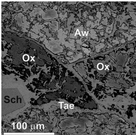
**Figure 1.** Awaruite (Aw) with oxide (Ox) products of alteration in taenite (Tae) matrix of Onello meteorite. Sch – schreibersite.
