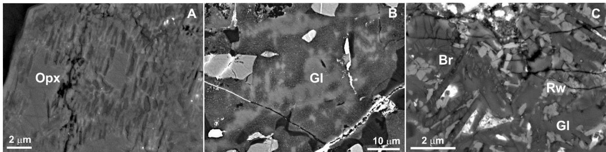
**Figure 1.** Orthopyroxene (Opx)-related microstructures in heavily shocked L6 chondrite NWA 5011: (A) Majorite-akimotoite aggregates replacing Opx; (B) Vitrified glass (Gl) after bridgmanite with akimotoite aggregates (dark areas); (C) Shock-melt vein background containing bridgmanite (Br), glass after bridgmanite and ringwoodite (Rw).
