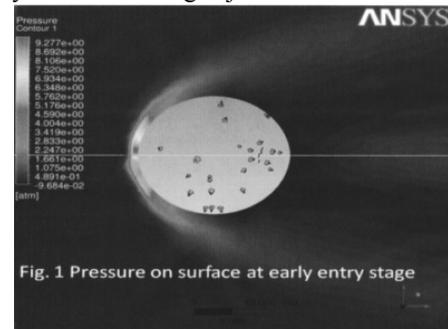
Fig. 1 Pressure on surface at early entry stage
