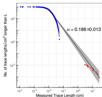
**Figure 1.** Distribution of flaw trace length for Bluff (a). The black line is based on the relationship between trace density and length, with a slope providing  $\alpha$ . The grey shaded area displays the error on  $\alpha$ .
