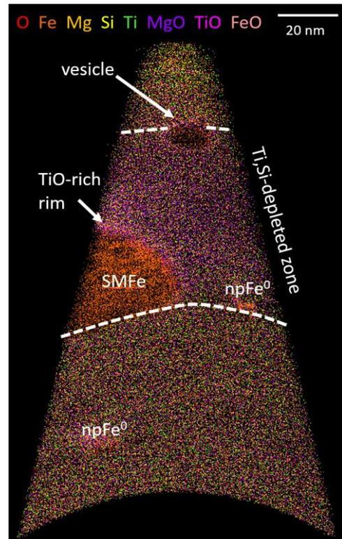
Figure 1: A 3-D APT reconstruction, in cross-section, of Tip C. Atomic or molecular ions are represented by a different color.
