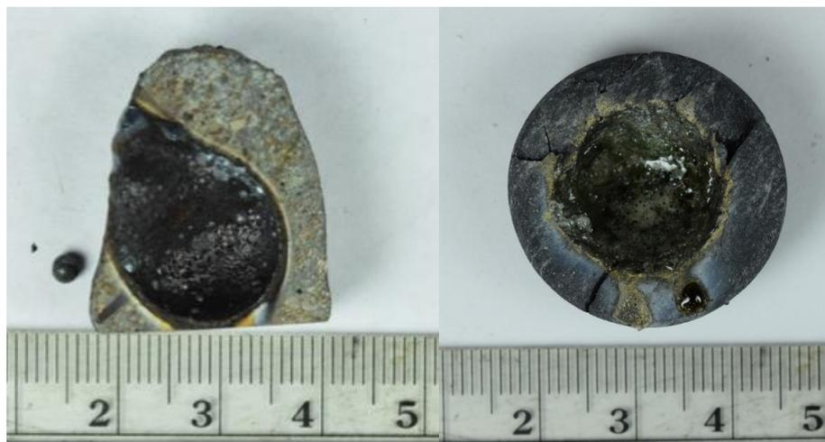
Figure 1. Tamdahkt chondrite and Basalt test models showing fusion crust and melt caused by laser testing.
