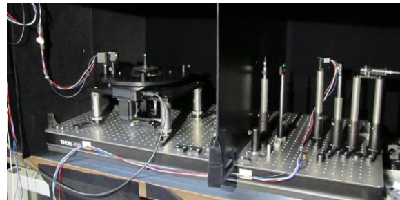
Figure 1: The scatterometer setup. The sample chamber is on the left, separated by a wall with a pinhole from the polarizers and beam shaping components. The leftmost wall has also a pinhole for forward light, and a beam dump behind the wall.
