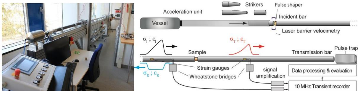
Fig. 1. Schematic setup of a Split-Hopkinson-Pressure Bar of the ALU-Freiburg
