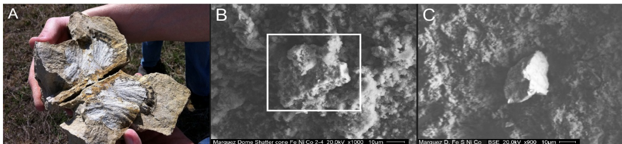
Fig. 1: Shatter cones from Marquez Dome, Texas. A: Freshly exposed, well developed shatter cone with reddish coating; photograph by David Rajmon. B: Kamacite aggregate on shatter cone surface, overgrown by sylvite, halite, and calcite (backscattered electron image). C: Fe-sulfide particle on shatter cone surface (backscattered electron image).
