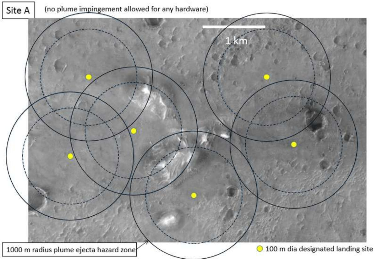
Figure 3. Example of Non-Interfering Landing Zones [4]
