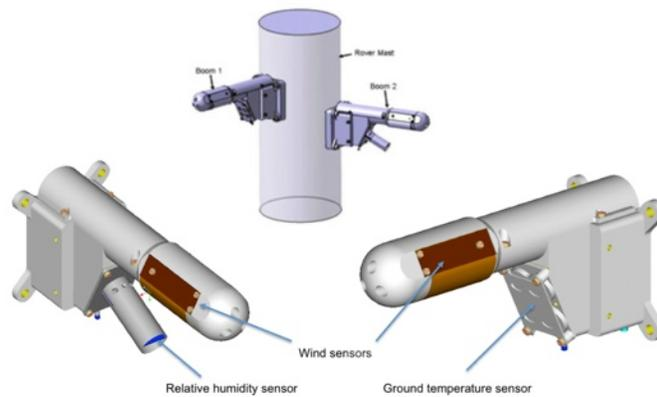
3. The REMS sensor booms, containing temperature (air and ground), humidity, and wind sensors, are attached to the mast of the Curiosity rover [6].
