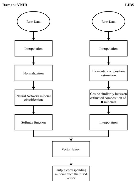
Figure 1: Simplified flow diagram showing our method for recognising minerals from combined Raman/VNIR and LIBS spectra.
