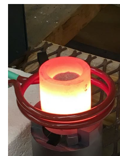
Figure 2: Magnetic induction based heating of a steel crucible run at 7.5 kW. Steel crucible reached a temperature of \sim 1500 °C.
