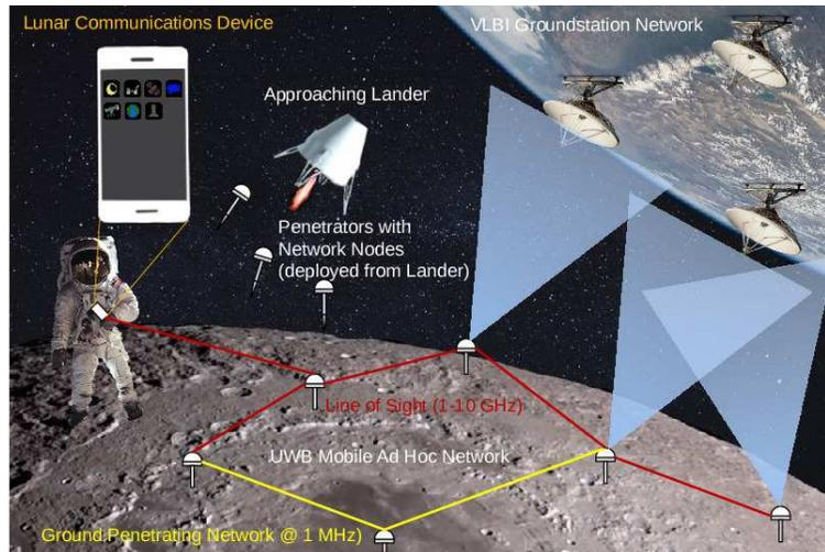
Figure 1: A LunaCell network set up to provide mobility and communications support for astronaut EVAs. This could include terminal landing navigation plus a LunaPhone “astronaut cell phone” for communications and PNT, both through a mesh radio network, and low frequency radio communications when out of line of sight of both the Earth and any other LunaCell node.
