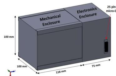
Figure 1: VEGA gravimeter layout
