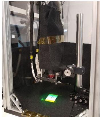
**Figure 1.** Image of prototype of AMIM instrument shown with green (525 nm) LEDs turned on. For scale, holes on optical base plate are  $\sim 1$  inch apart.
