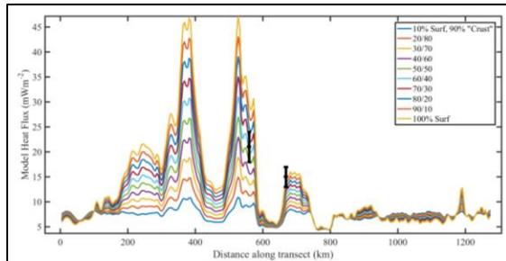
**Figure 4: Forward model of possible global heat flux along transect line in Figure 3 showing that Apollo sites poorly constrain crustal composition.**
