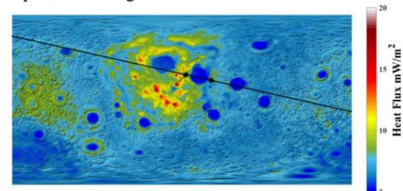
**Figure 3: Forward model of possible global heat flux based on the surface Th representing 10% of the crust.**
