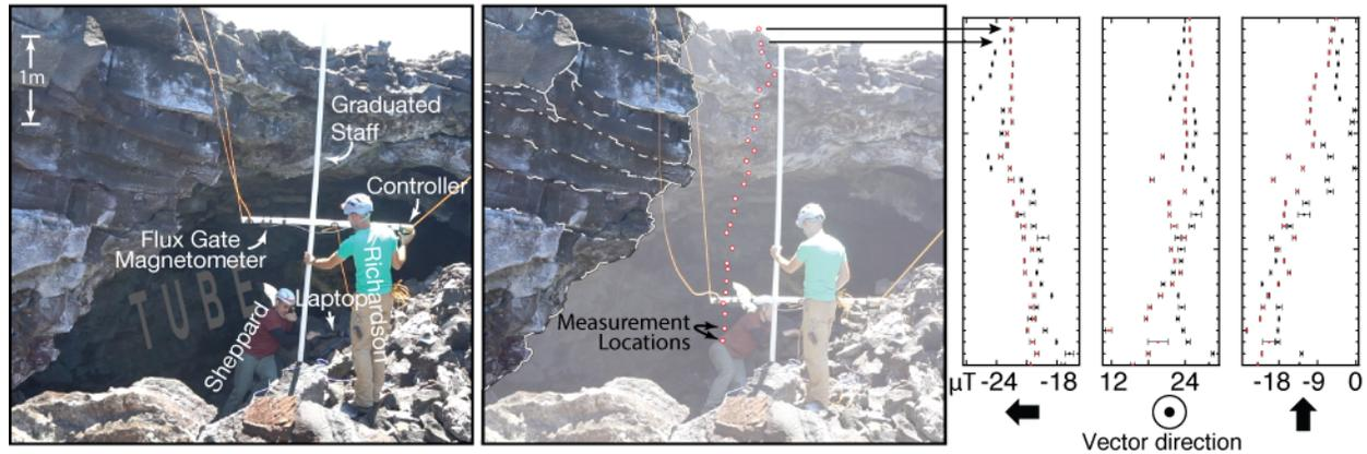
Figure 2. We used a 3-axis fluxgate magnetometer to survey a vertical lava flow cliff on Mauna Loa, Hawaii. A similar investigation on the Moon will enable examination of magnetic properties of different lava flow layers.
