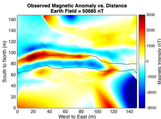
Figure 3. Magnetic anomaly maps can help identify buried structures like lava tubes. Skull cave (LBNM) produces a negative anomaly. The gradient of the magnetic field helps identify cave boundaries.
