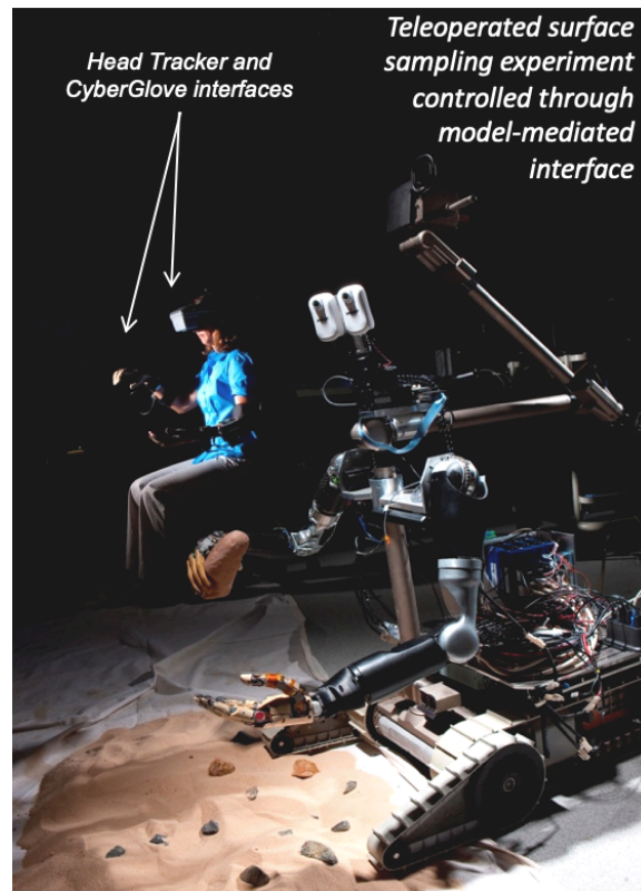
Figure 1. Allie on Earth controlling ALLIE on the simulated surface of the Moon. Concept only. We propose to develop the architecture addressing design, control, and operation.
